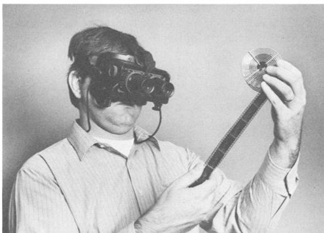
FIG. 8—Stripping the film from processing reel for subsequent inspection. Note the use of the Litton AN/PVS-5A Nightvision goggles.
